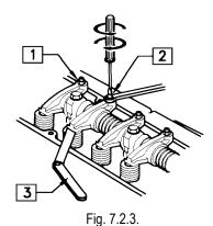
After the adjustment, the rocking nut should be well tightened while the adjusting screw is locked so that it does not rotate.
