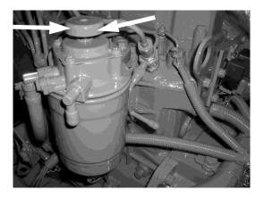
(3) Engine equiped with fuel puma type VE, bleeding the air pushing the button of the fuel filter (showed in the photo). The air bledding from the injection puma and the injectors is automatic.
