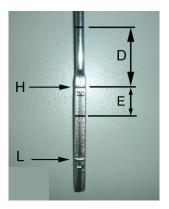
When the engine is fitted inclined, the oil dipstick must be modified to avoid problems of aspiration by the oil pump. See the table enclosed for modification level in rod oil. Increase level D or decrease the level E (depending type engine), starting off of level H of the original oil dipstick.
