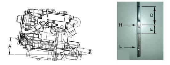
When the engine is fitted inclined, the oil dipstick must be modified to avoid problems of aspiration by the oil pump. See the table enclosed for modification level in rod oil. Increase level D or decrease the level E, starting off of level H of the original oil dipstick.
