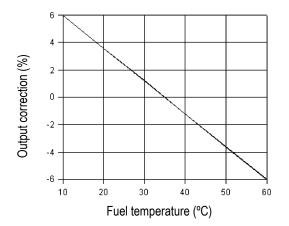
Graph 1 Effect of fuel temperature on engine output. +35°C is reference temperature (0%)
