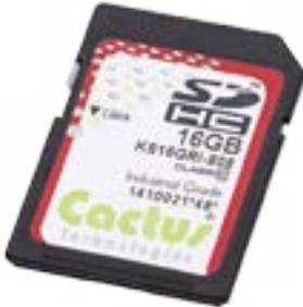
The Cactus Technologies Secure Digital Memory Card (SD) - 808 Series is a low capacity solid-state flash memory product that complies with the Secure Digital Card Association (SDA) standard. Cactus SD Cards provide up to 16GB (Class 10) of formatted storage capacity and are designed to be used in applications which require reliable, high performance solid state storage in a small form factor.
