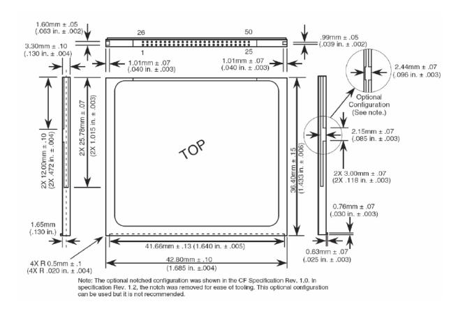
Figure 2-1. CompactFlash Memory Card Dimensions
