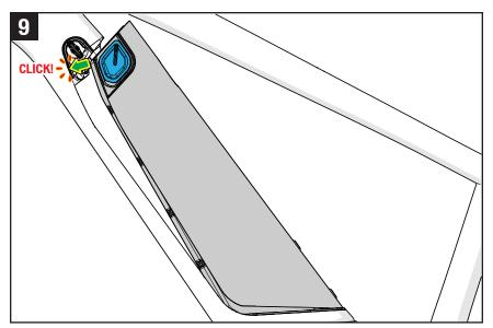
Press down on the battery near the power button until it clicks and engages with the lock (fig.9).
