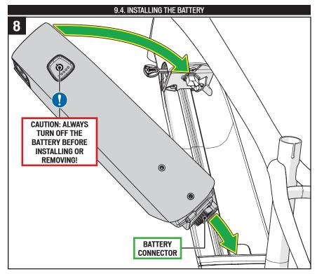
Lower the bottom edge of the battery into the bottom of the battery cavity (fig.8), then align the top of the battery with the top of the cavity.
