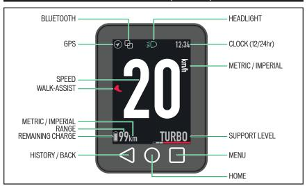
The display is controlled using the buttons on the handlebar remote (fig.4), as well as the three touch buttons below the display and the touch-enabled display itself. The touch screen can be navigated using touch, swipe, pinch and spread gestures.
