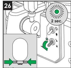
The keg is now locked and the pump audibly generates positive pressure in the keg. Once the pump switches off after around 30 seconds, the beer is cooled actively. The cooling fan is the only thing that can now be heard.
