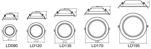
The minimum distance from the top of the luminaire to any normally flammable building element is 40 mm.
