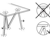
For optimal stability, Accordion should thouch the tabletop and the floor on all points. This can be achieved by moving the legs a little in the direction the dashed arrows indicate.
