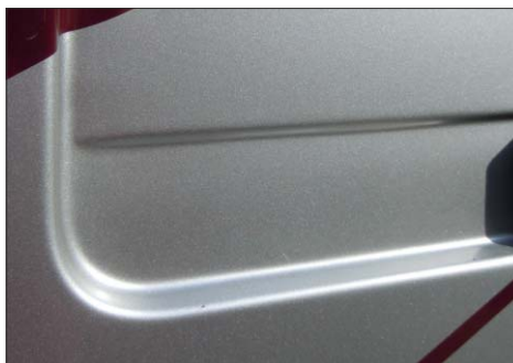
SOTT ADHESIVE ACTIVATOR 600-AA1400 helps in those spots where the film remains under tension. The primer reduces the surface tension of the substrate and consequently improves bonding with the adhesive.
