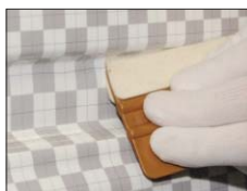
Don't forget to re-squeegee after heat-setting. There are various ways to do this, but what matters is that the film is pressed onto its substrate once more.
