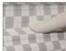
Don't forget to re-squeegee after heat-setting. There are various ways to do this, but what matters is that the film is pressed onto its substrate once more.
