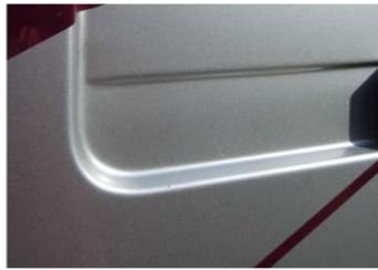
When signing or when wrapping a car, you will always have to deal with sharp edges and deep grooves, where normally the film would thin out and could discolorize or deviate from the original. This simply can be solved by shifting and spreading the film tension.
