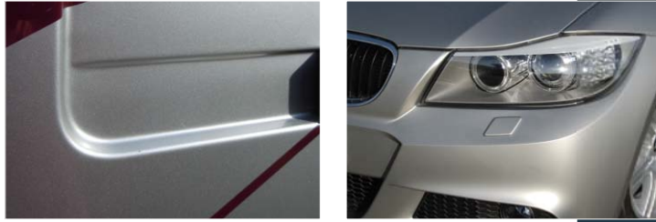
When signing or wrapping a car, you will always have to deal with sharp edges and deep grooves, where normally the film would thin out and could discolorize or deviate from the original. This simply can be solved by shifting and spreading the film tension.
