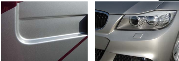
When signing or wrapping a car, you will always have to deal with sharp edges and deep grooves, where normally the film would thin out and could discolorize or deviate from the original. This simply can be solved by shifting and spreading the film tension.
