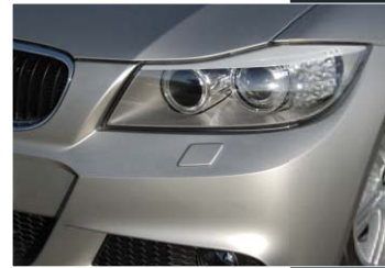
When signing or when wrapping a car, you will always have to deal with sharp edges and deep grooves, where normally the film would thin out and could discolorize or deviate from the original. This simply can be solved by shifting and spreading the film tension.
