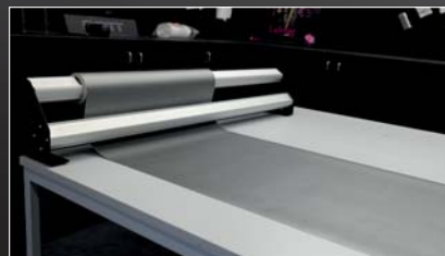
The two aluminium roller guides enable you to unroll your vinyl or application tape either from the top or the bottom.
