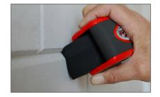
In this image you can see that the hard foam wheel easily takes the shape of the curved surface.
