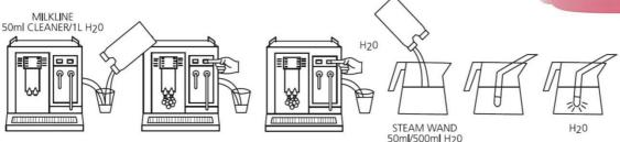
Ensure the white cap is tightly sealed and slightly loosen the red cap. Gently squeeze the bottle until reservoir measures 50ml, remove the red lid and pour from reservoir. Cleaning Milk Frother:
