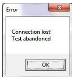
Once the message has been acknowledged, it will be possible to select control buttons and menu options in the Otosure window on the PC but these will have no effect. If the Otosure cable becomes disconnected, the recommended course of action is for the operator to close the Otosure window and return to Audibase. Then use the "Edit > Cancel Insert/Edit" option or cancel toolbar button to remove any data, and close Audibase. The Otosure may then be reconnected and Audibase started as usual.
