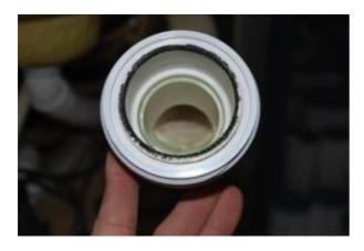
The O-rings are still totally clean after use of AquaFinesse. There is no sign of damage. The sealing rings below have been used since 2004.
