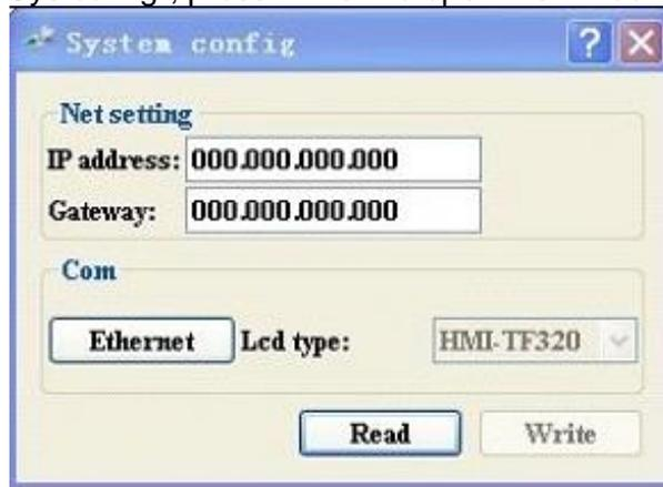
By default, the cursor is on the "Read" button. Press "Enter" to retrieve the information. The "Z+/-" keys can be used to alternate between the information. Information that has changed can be stored by selecting "Write" and pressing "Enter". "Lcd type" cannot be changed. You can press "Ethernet"/"USB" in the section "Com" to open the selection window between connections. This screen needs a password to get in and can be provided by BRM.
