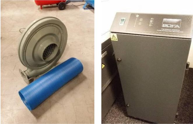
The extraction unit or Bofa can be connected to the laser via the air outlet in the centre/rear bottom of the machine by means of the included hose. The electrical supply for the extraction unit or Bofa is provided by a socket (EU 230/240V 50/Hz) in the rear of the machine.
