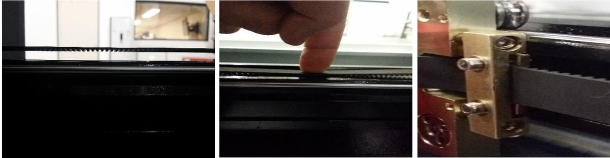
As for the x-axis, you cannot check if it is suspended. In other words, pull it carefully towards you until you feel a bit more resistance. Then you measure the distance to the line. This must be maximum 30 mm. If this is a lot more, that means the belt is loose. And just like the y-axis, afterwards push the belt with your finger against the line.
