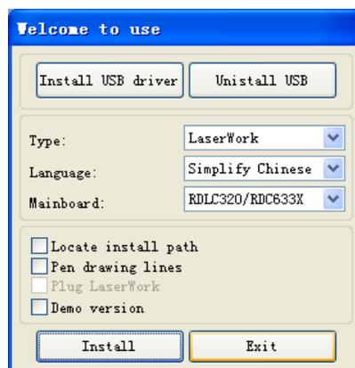
Use the top 2 buttons to install or uninstall USB-drivers. These must be installed first before you are able to proceed. After this installation, you will notice a window with options to select the software.
