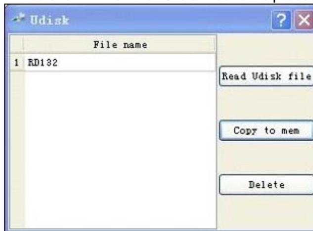
The system now show all the files on the USB-stick when it's connected. The USB-stick must be FAT32 formatted and not be larger than 4 GB. The programmes must not be in folders on the stick. When copying from the machine to the stick, it will also be copied to this location.
