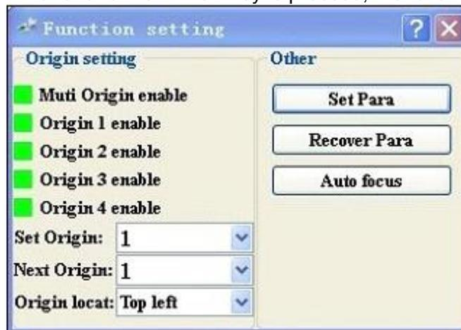
You can change the status when the cursor is on "origin x enable" and "Enter" is pressed. Red is on and green is off in these fields.
