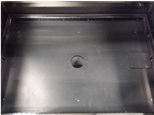
The waste tray must be kept clean. Cut material is flammable and too much cutting material can ignite due to the heat of the beam. The port of the extraction unit must be kept clean to guarantee proper reduction of laser gases.
