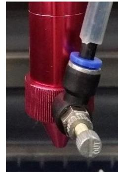
The air pump receives its power from the socket at the rear of the laser machine. The connection for the air supply can be found there as well. The air will be brought inside the machine towards the laser head when the compressor is connected to the socket and air supply. The laser head is equipped with a valve to adjust the quantity of air. Experience has shown that adjusting the setting of the valve produces a better result.
