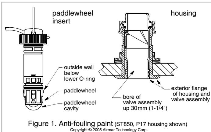
Figure 1. Anti-fouling paint (ST850, P17 housing shown)
