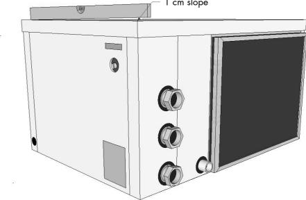
The unit should be mounted in such a way that the side of the condensation drain is at least 1 cm lower than the other side (slope) to ensure that the condensate drains properly. In practice, the 1 cm elevations at all corners – except the corner of the electrical compartment – are exactly right for a correct fall. Using a spirit level is recommended.
