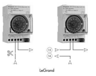
The two ends should be connected to terminals 15 & 16 on the terminal strip in the electrical compartment of the OptiClimate.
