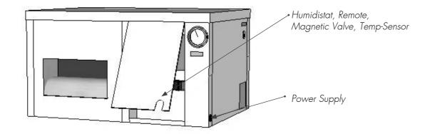
First, the panel at the left side near the manometer should be removed to make the various electrical connections. A water valve, water leakage sensor, automatic moisture meter, remote control and room temperature sensor are supplied with the unit. Their cables can be led to the outside through the opening at the bottom of the panel. The power cable for the power supply can be led through the black feed-through rubber at the side of the unit.
