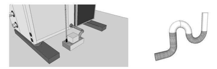
Drain pump of the condensation water
