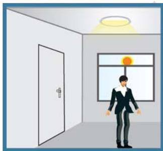
The lamp dims to minimum light level but never turn off even if with sufficient ambient light.
