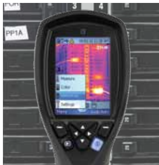
FLIR i3, temperature in 3,600 spots
