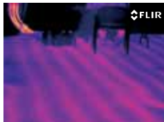
Leaks in an underground district heating network.
