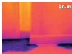
Moisture intrusion in floor, impossible to see with the human eye, but clearly visible in the thermal image.
