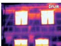
Framework construction. Many of the sections are missing insulation as indicated by the warmer colors.
