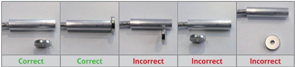
If the magnet is located close enough to the proximity switch, the switch closes. If the magnet moves away from the proximity switch when the trap doors close, the trap alert triggers an alarm.
