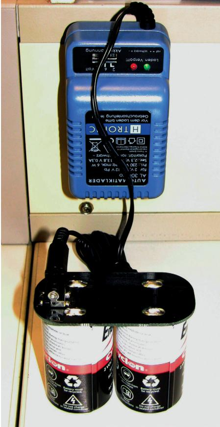
The TRAPMASTER is supplied with a special rechargeable battery. This battery is designed for a very wide temperature range (down to  $-40^{\circ}\text{C}$ ), in order to ensure reliable trap monitoring even at prolonged minus temperatures.
