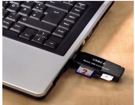
Disabling the PIN with an old mobile phone Alternative: USB SIM card reader
