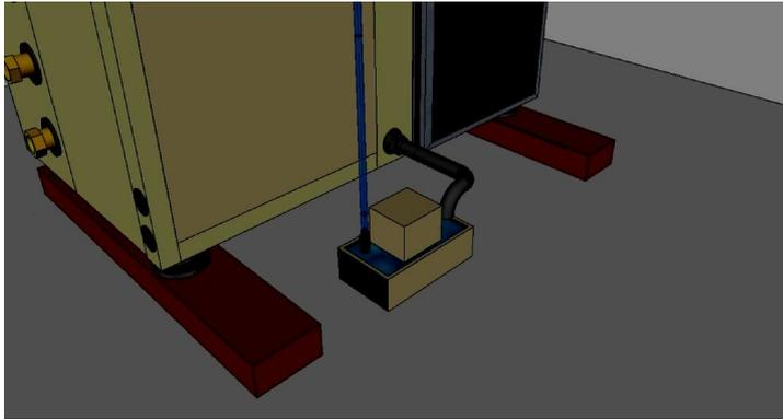
*Drain pump of the condensation water installation*
