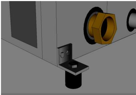
*Installation of insulating springs*
