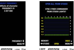
**RIGHT JOYSTICK:** use the UP / DOWN arrows to scroll through the frequency options
