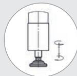
Pivoting foot with sturdy M30x2 (System D28), M28x2 (System D22) or M24x2 (System D16) threaded spindle, adjustment travel 30 mm fine adjustable.
