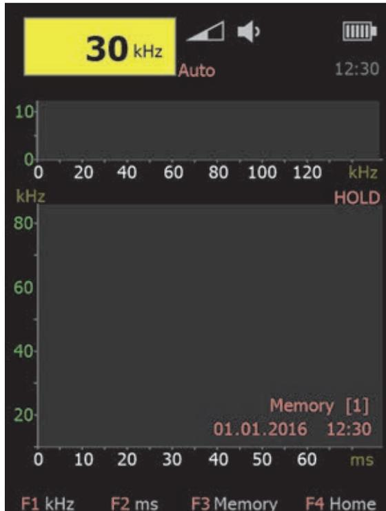
By pressing the button F3 in the mode-submenu you get to the **sonogram-submenu**
