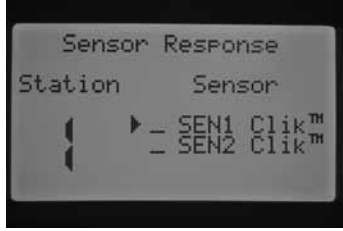
No sensor programmed for Station 1
