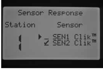
Sensor 2 only programmed for Station 1
