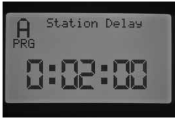
EXP: STATION DELAY FOR PROGRAM A 2 MINUTES
