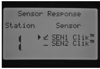
Sensor 1 only programmed for Station 1
