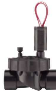
PGV-100JT-G Inlet Diameter: 1" Height: 5½" Length: 4½" Width: 3¼"
