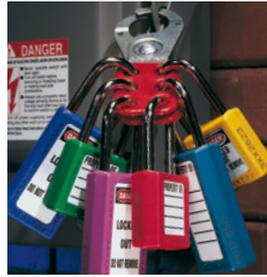
Lockout hasps are an integral part of a successful safety lockout program, providing effective multi-person lockout :
