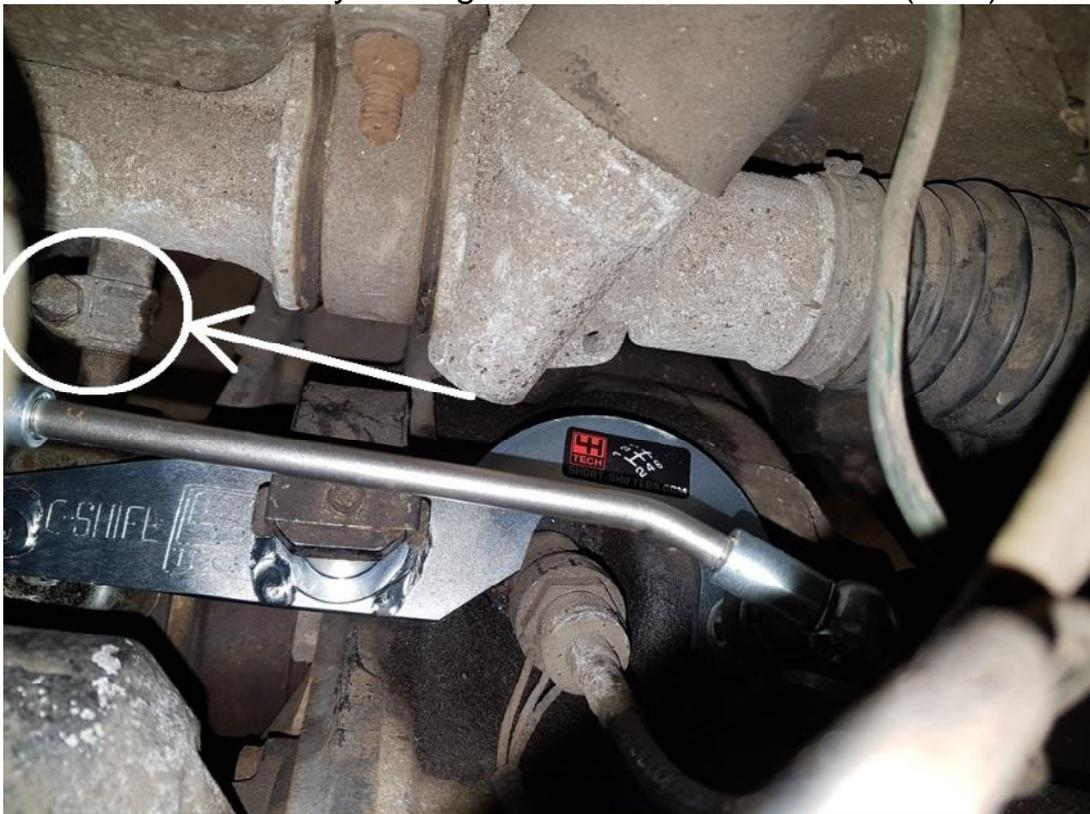
Put the new shifter back in the car. Fit everything in reverse order, but wait with tightening the bolt which connects the shifter with the shift lever bar.
