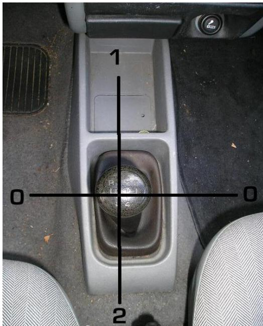
Keep the gear lever in the neutral position against the left side and keep it in this position.
