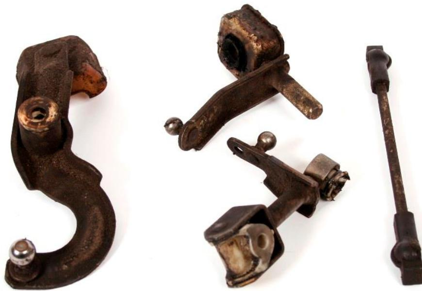
Remove all single shifter parts from the OEM shift linkage.
