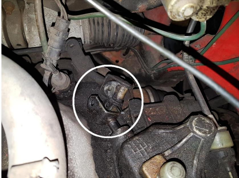
Remove pin between gearbox and shift mechanism
