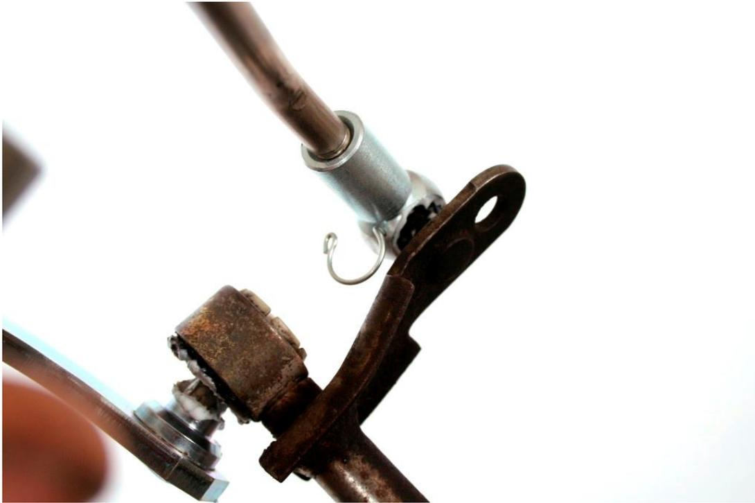
Don't forget to secure the new top shifter bar with the new pins, like shown on this picture. Put the pins in the little holes of the bolt head, and secure them by turning them over the bolt head. (click)
