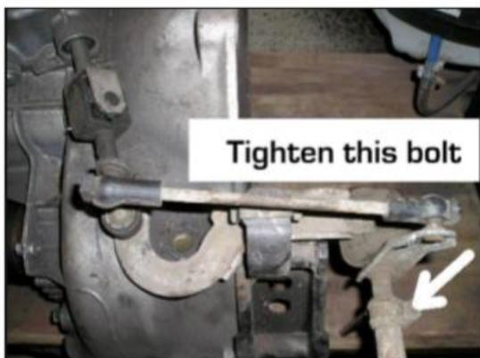
Ask someone to keep the lever in this position and tighten the bolt.
