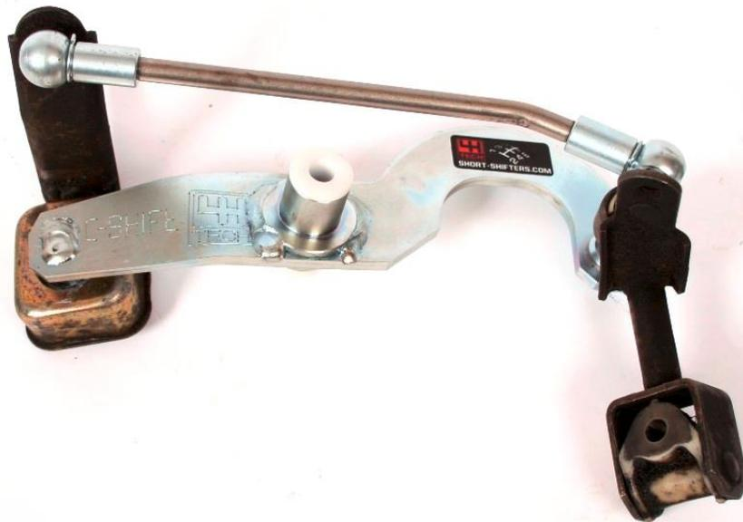
Fit all parts to the new shifter arm, and use the new shifter bar on top, and fit the new nylon bushings
