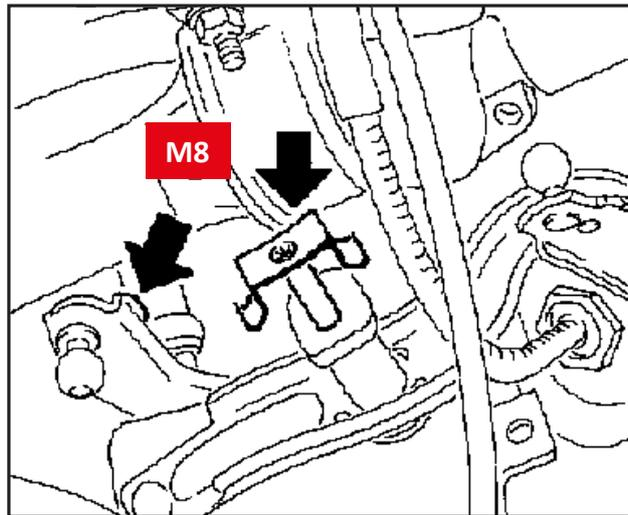
Dismantle the old linkage complete and reassemble every part on the new linkage (shift shortener). When reassembling, fill everything with silicone grease before fitting to be sure of a smooth gearchange.
