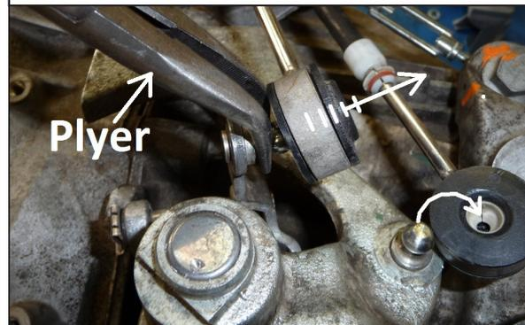
Remove cables from ball joints.
