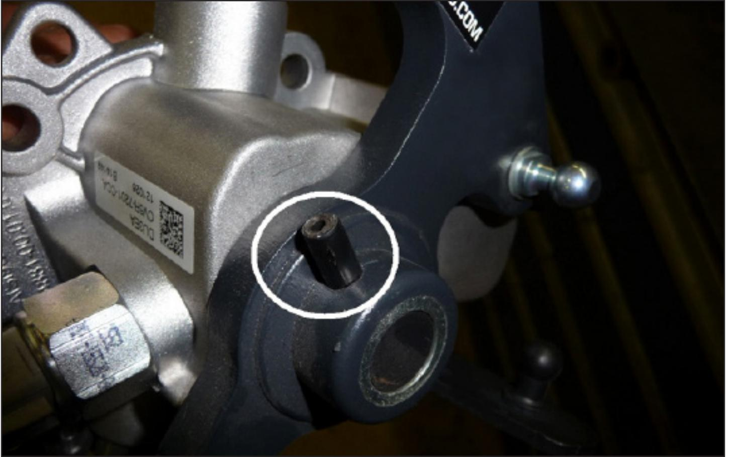
Use the old pin to secure the new Short Shifter arm to the shaft of the shifter unit. You can use the punch and a hammer again to tap it in to place.
