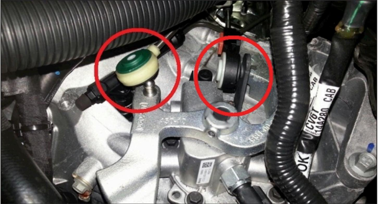
Unclip both shift cables by putting a 13mm spanner between the cable head and the shifter arm.
