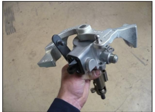
Unclip the connector from the shift unit, and remove the bolts which secure the shifter unit to the transmission. (4 bolts) The shifter unit can now easily be pulled straight out of the gearbox.
