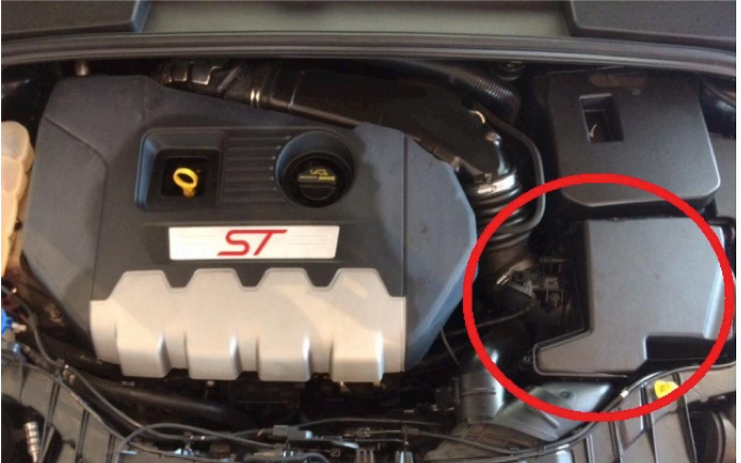
Open the bonnet, and remove the air intake hose and airfilter box .
