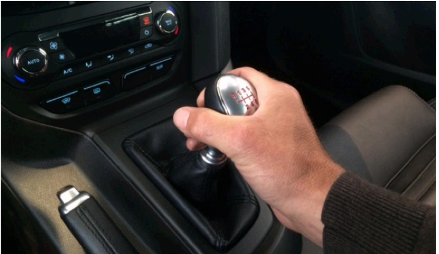
Put the gear selector in neutral position.
