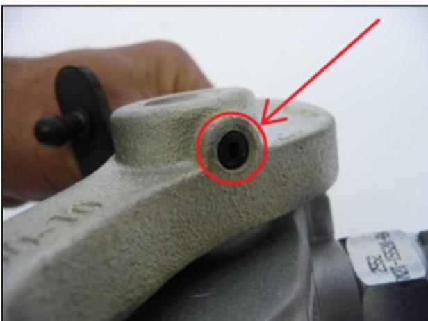
The original shifter arm is secured on the shaft with a steel pin. This pin can not be removed with the shifter still in the engine bay. For this reason it is necessary to remove the complete shifter unit.
