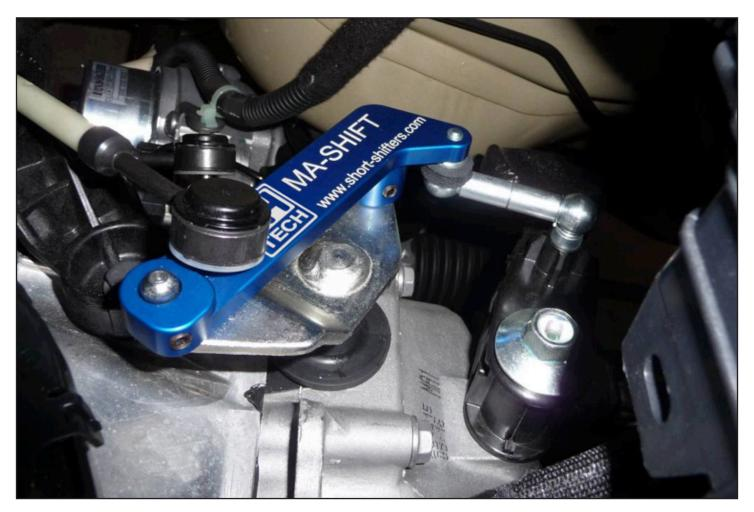
Fit everything back in the car (air cleaner) Check if all gears can be engaged, and take the car for a test drive. 35% shorter gear throw.
