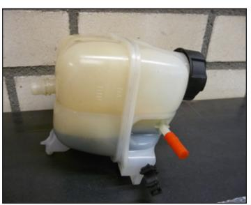
Pull up the cooling tank and detach the bottom hose. (pull back clip). Put the white plug (supplied with the kit) in the hose connector to avoid cooling water coming out. Store the cooling tank like shown on the picture. This way no cooling water wil be spilled at all.
