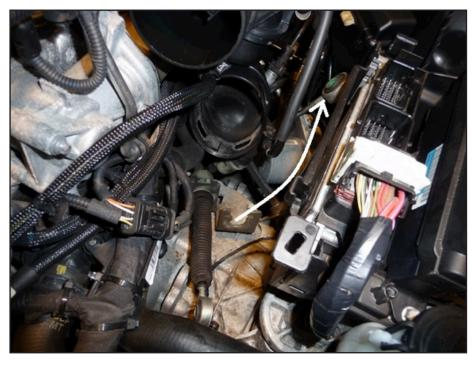
Detach the right shifter cable from the bracket, and put it aside.
