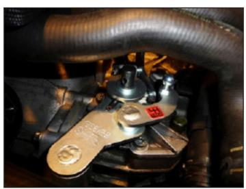
Put the supplied new pin in the new shifter arm and tap it further till it sits just free of the inner side. (see picture). Put both shifter arms on the gearbox, before tapping the pin further in it. (this way the shifter arm can still be turned every side to fit all other shifter parts easy.)
