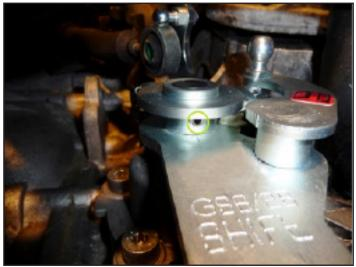
Now tap the new shifter pin further in it. (you can put the shifter in a gear which causes the arm to be in the lowest position. The new pin is easy to fit, you do not have to use much force to get it in position)
