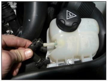
Open the bonnet, and remove the top cooling hose from the reservoir. Parts from this kit can be used to remove the reservoir without cool water coming out anywhere. Very easy!
