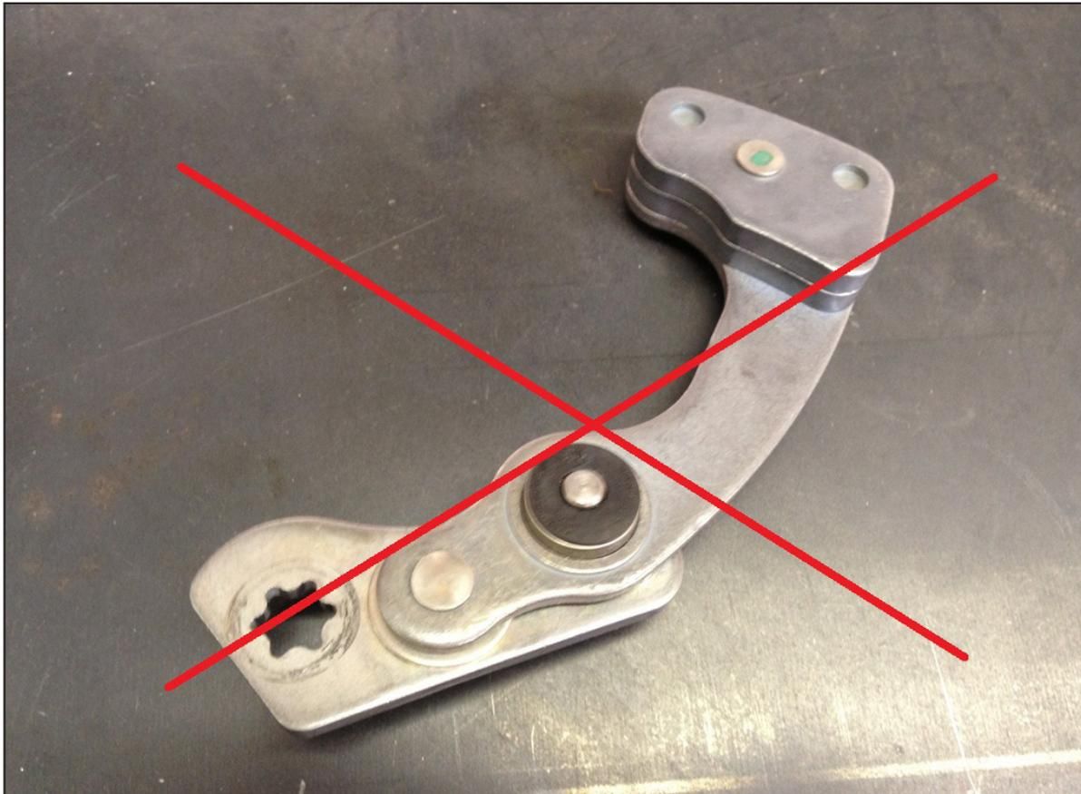
**Pull the old shifter from the shaft. (it can be done by hand, but can be very stuck in some cases)**
