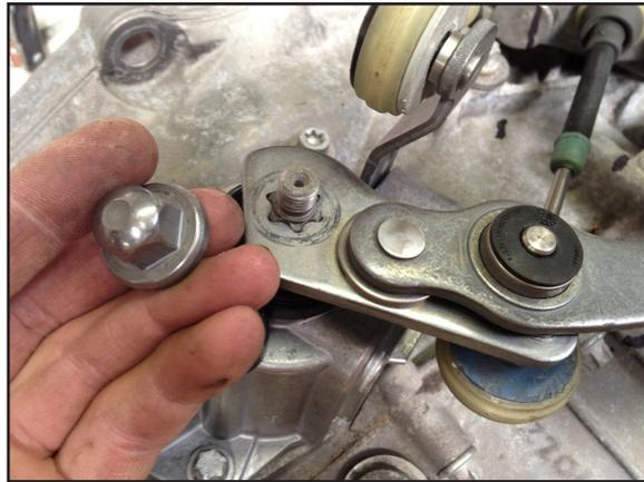
**Important: support old lever with your hand while removing the nut!**
