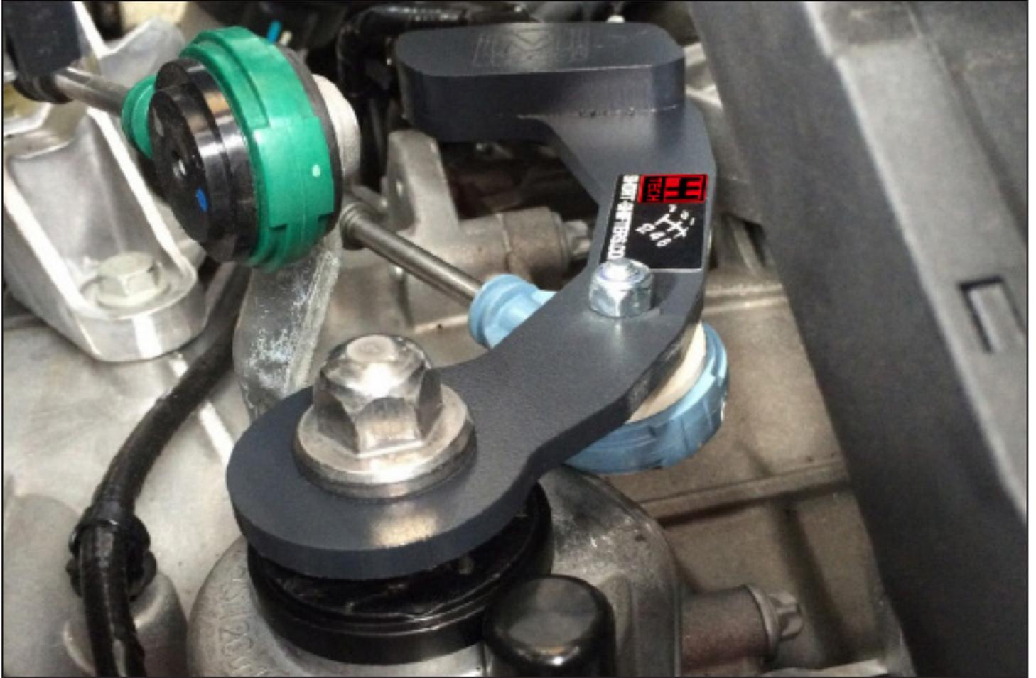
Click on the shift cable first, before mounting the shifter.
