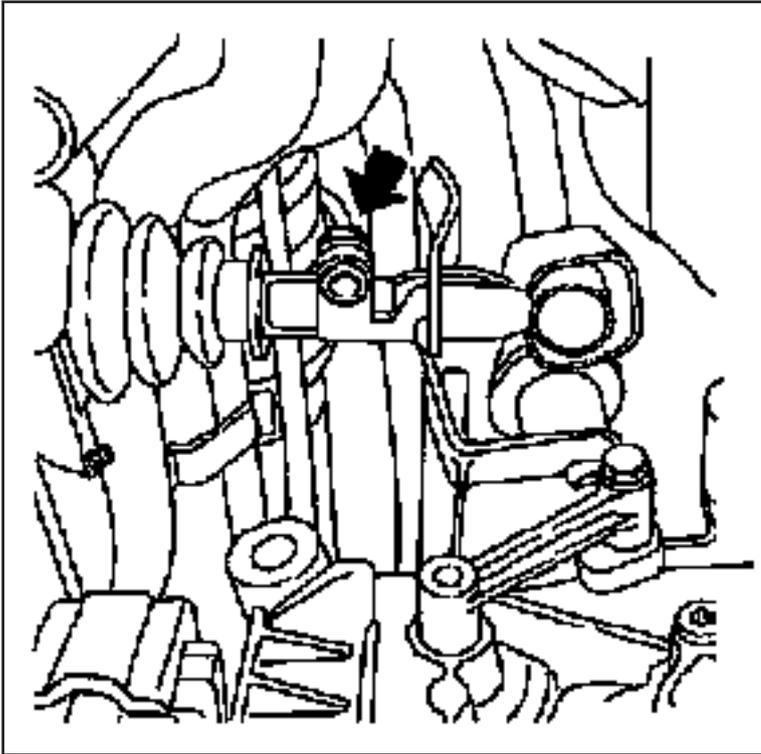
Pull the adjustment pin back out of the casing. Check that all gears can be engaged satisfactorily. Refit the gear lever boot.
