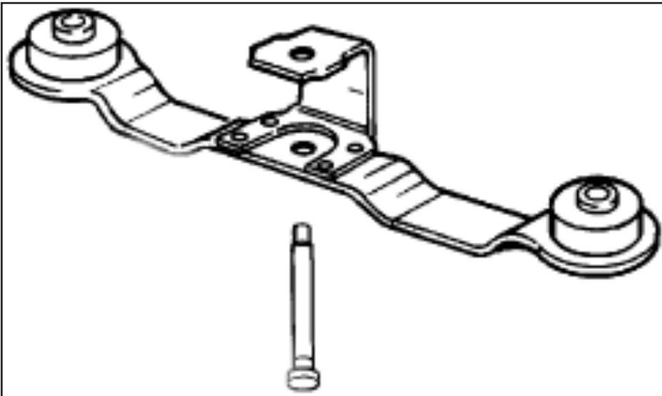
**Dismantle the old linkage complete and reassemble every part on the new linkage (shift shortener)**
