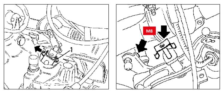
**Dismantle the old linkage complete and reassemble every part on the new linkage (shift shortener)** When reassambling , fill everything with silicone grease before fitting to be sure of a smooth gearchange.
