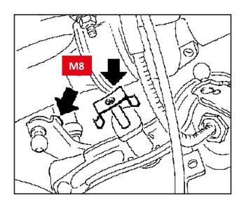
Dismantle the old linkage complete and reassemble every part on the new linkage (shift shortener). When reassambling, fill everything with silicone grease before fitting to be sure of a smooth gearchange.
