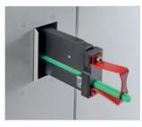
Perforating and creasing tools The tools are automatically detected and the relevant pressure is automatically set. Additional tools may be stored in the especially designed parking slots.
