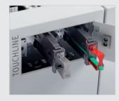
Two cross tool positions The creasing and perforat-ing tools are automatically detected and the relevant pressure is automatically set. No manual adjustments are needed.
