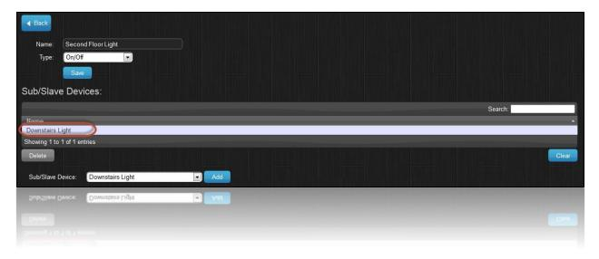
\*Note: When adding a Sub/Slave device, this will not be visible in the 'Lights' tab by default. You see this device in the 'Edit' screen from the device you added it too.
