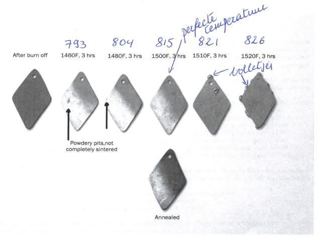
7. After you have determined the ideal temperature, fire another piece exactly the same way at the ideal temperature. After firing anneal this piece using the following procedure:
