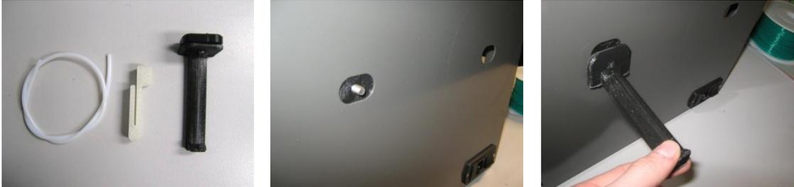
6. Remove the plastic from the filament and place the role on the Filament arm. Now feed the filament thru the clip and tubeing.
