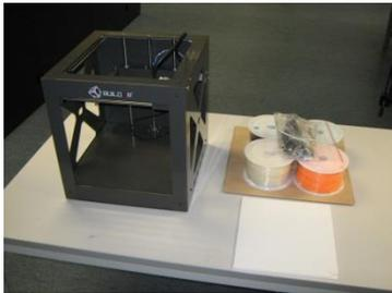
3. Remove the foil from the print-tableau. Place the Tableau in the machine fitting the corners on the screws in every corner. Make sure to press down making sure the tableau is all the way down on the screws
