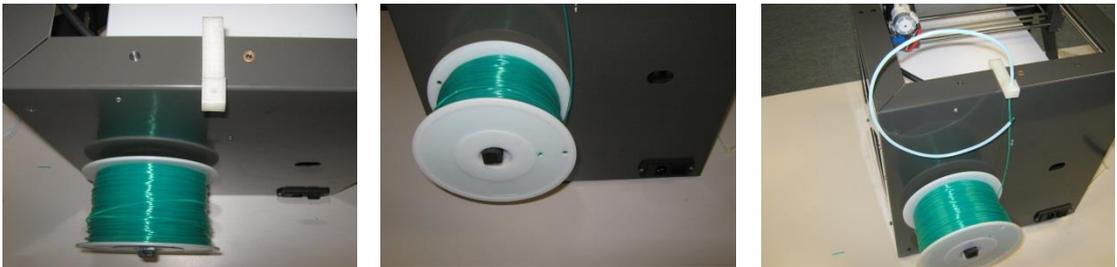
7. Feed the filament thru the tubing until it reaches the extruder. Open the lid of the extruder by squeezing the spring-screws. Feed the filament all the way into the extruder. Close the lid and make sure the spring-screws return in the correct position.
