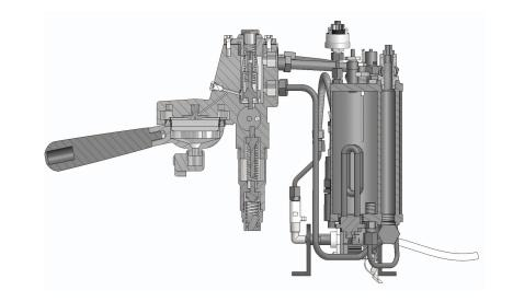
The large rectangle represents the case of the Vibiemme espresso machine. It houses all the mainly working elements of the machine as shown above: Boiler , Boiler pressure gauge, Brew gauge and Grouphead.
