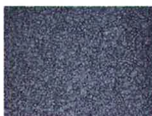
Alumina – BIO-HIP Grain Size 1.8 \mu\text{m}
