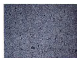
Alumina – status 1980 Grain Size 4.0 \mu\text{m}
