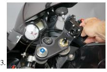
The StemMount is designed to snugly fit into the steering stem hole, in the top triple clamp assembly. If your bike has a rubber plug in this hole, it must be removed.
