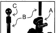
**10.** Attach double ball and socket components and adjust to desired position to complete assembly.
